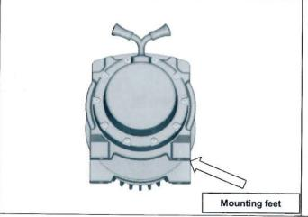
Before installing the winch make sure the clutch handle is opposite the mounting feet as shown (usually as supplied new in box).
