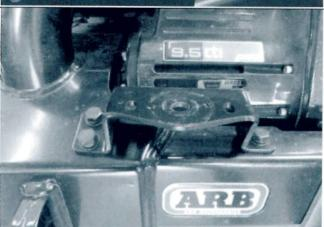
If driving lights are to be used fit left and right driving light mounts now using M8 x 25 bolts, M8 spring washers, M8 flat washers and M8 flange nuts.
