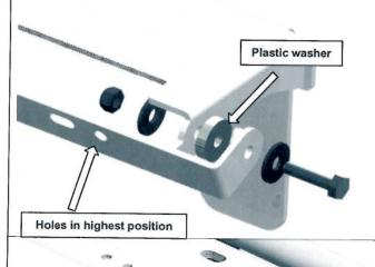
13. Assemble pivoting license plate bracket as shown. Place plastic washer between holder and bracket and secure using M6 x 25 bolts, flat washers and M6 Nyloc nuts. Make sure license plate holes in pivoting bracket are in the higher location.
