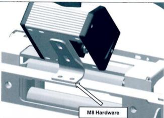
15. If mounting a control box on the bar secure mount to bar using M8 x 25 bolts, M8 spring washers, M8 flat washers and M8 flange nuts. Secure control box to bracket using manufacturers' hardware.
