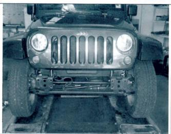
This is how the vehicle must be prepared before fitting a bar to the vehicle. Wrap up and cable tie fog light wiring out of the way.
