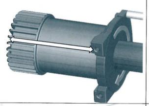
If fitting a winch measure the distance between winch mounting hole and the end of the motor. If this distance is greater than 172mm than a notch in the chassis flange must be cut. Follow step 4.
