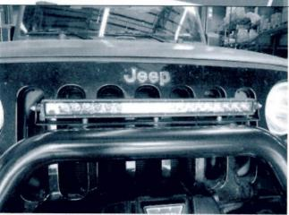
The top tube mount can be used for LED light 16. bars or fitting of radio aerials.
