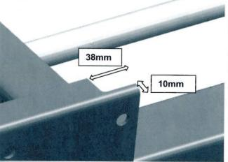
Measure from front of chassis back 10mm and mark a line. Measure from inner edge towards chassis centre 38mm and mark a line. Cut this section out using a grinder with cutting disk, de burr and paint.
