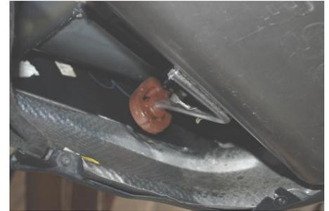
4. Be sure hanger is correctly installed into the rubber grommet for complete support.
