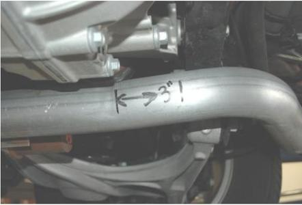
2. To remove the factory exhaust measure from the rear bend 3" forward. Please reference picture for location. Mark and cut with a hack saw or cut off wheel. Leave the factory rubber grommets in place they will be re used.
