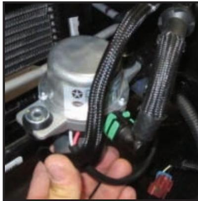
Step 6: If needed a Zip Tie can be used to pull air lines together.
