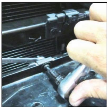
Step 11: Inspect all air lines and wires. If needed Zip Ties can be used to position lines away from plate.
