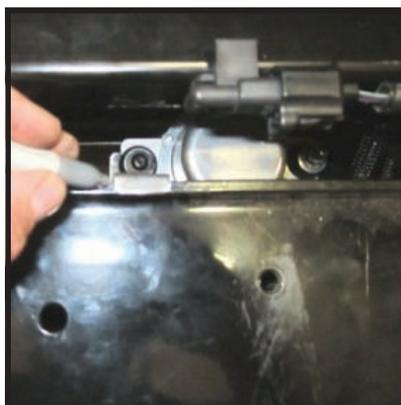
Step 9: With plate removed from frame and mounting hole marked drill 1/4" hole into winch plate. Apply black paint to exposed metal.
