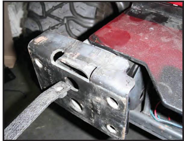
3. Insert a M10 hex bolt and M10 washers thru the hole of the winch plate and frame threading into the nut plate. Tighten. Repeat for opposite side.
