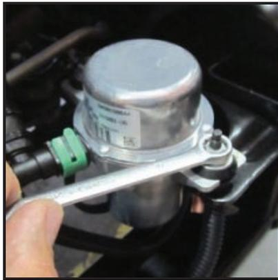
Step 2. Remove front bushing from pump and flip over as shown. Tall side will need to face up. Reinstall bushing.
