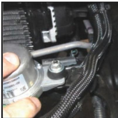
Step 5: Disconnect small air line and wire harness. move harness and hose to the front of pump. Reconnect.
