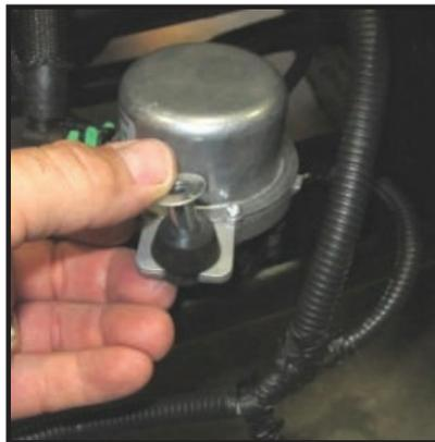
Step 3: Rotate pump as shown. Front mounting tab will be relocated to factory rear mounting stud.
