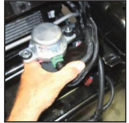
Step 4: Secure pump to rear factory stud using M6 nut removed in step #1.
