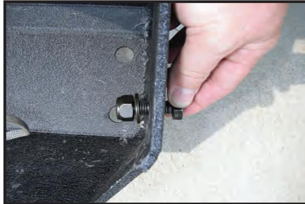
2. Insert a M12 hex bolt and washer thru the top holes in the stubby end. Install the stubby end onto the bumper by sliding the notch cutout on the lower portion of the end onto the bottom bolt. Line up the top bolts with the bumper and insert them into the bumper fastening with a hex nut and washer. Tighten all bolts. Repeat for opposite side.
