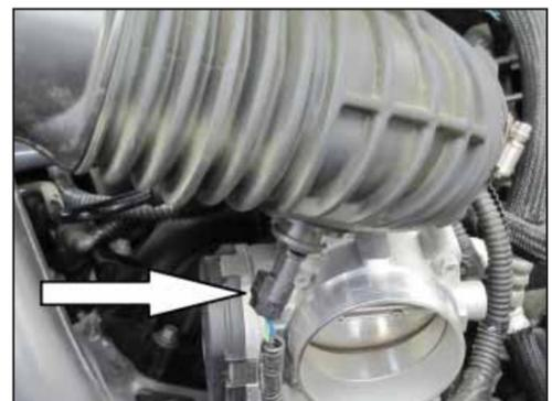
6. Lift up the intake tube and then disconnect the inlet air temperature electrical connection. Then remove the intake tube from the vehicle.
