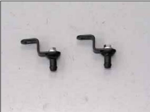
11. Install the two provided mounting studs onto the two heat shield brackets (070061) as shown
