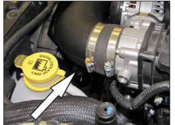
33. Reconnect the inlet air temperature sensor electrical connection
