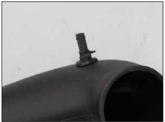
28. Install the provided grommet and factory inlet air temperature sensor into the K&N intake tube as shown. **NOTE: Be sure to remove the O-ring from the sensor before installing it into the grommet.**
