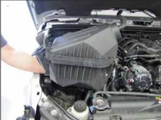
8. Lift up and remove the air filter housing from the vehicle.
