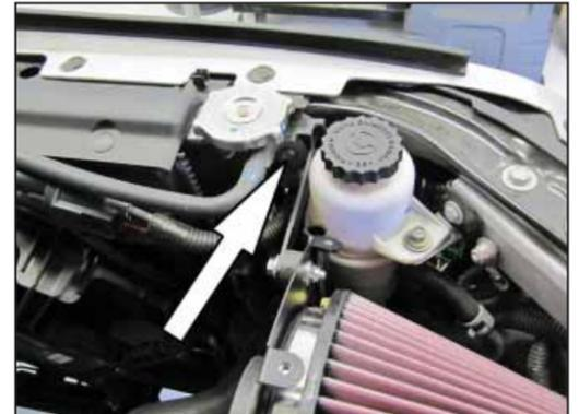
19. Install the heat shield bracket assembly onto the heat shield and radiator mount as shown. Secure the bracket with the factory bolt in step # 9 and the hardware provided.
