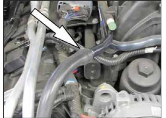
32. Connect the open end of the crank case vent hose to the factory crank case vent tube as shown.
