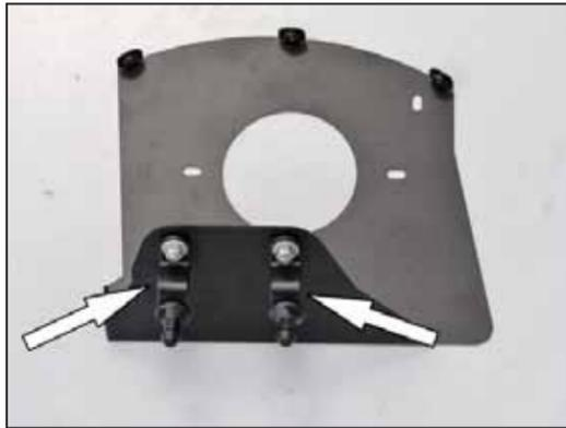
12. Install the two heat shield bracket assemblies onto the heat shield as shown.
