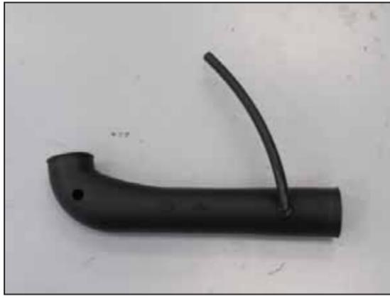
26. Install the provided crank case vent hose onto the fitting as shown.
