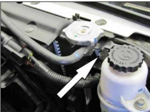
10. Remove the bolt show that secures the radiator to the core support.
