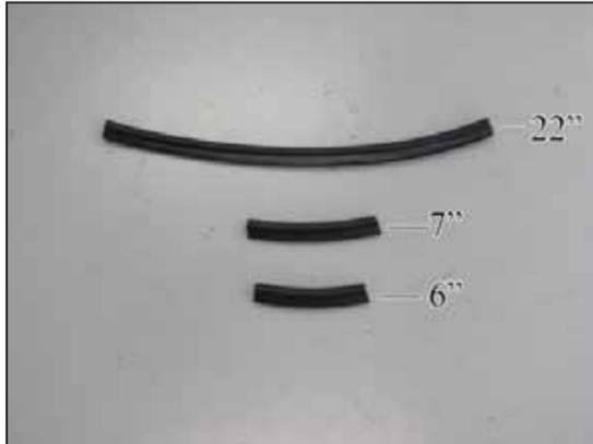
14. Cut the provided edge trim into three sections. One section is to be 6" long, one section is to be 7" long and the final section is to be 22" long.
