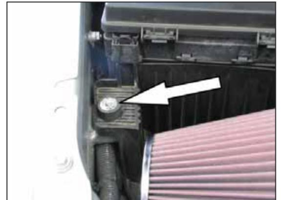
20. Install the rubber mounted stud into the into the air box mounting plate bolt location as shown.
