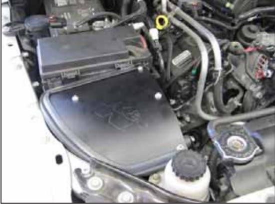
22. Install the K&N filter lid and secure with the provided hardware. **NOTE: Start the bolt into bracket (083163) first.**
