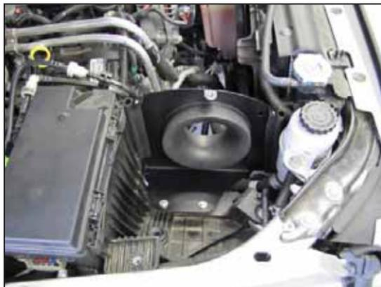
16. Install the heat shield assembly into position so the mounting studs are in the air box mounting grommets.
