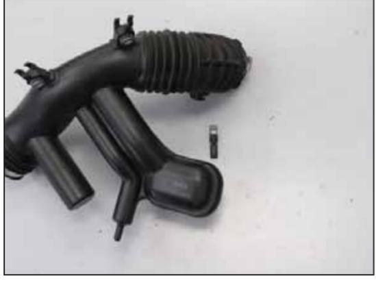
27. Remove the inlet air temperature sensor from the factory intake plenum as shown. **NOTE: Use caution working with the inlet air temperature sensor as it is very fragile.**
