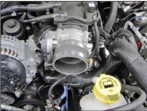
24. Install the provided silicone hose (08690) onto the throttle body and secure with the provided hose clamp.
