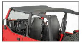
Important: For a smooth fit and ease of installation, this top should be installed at temperatures above 72 degrees. Below this temperature, the fabric may contract an inch or more making it difficult to install. We highly recommend taking the top out of the package and letting it sit inside a warm place or direct sun light for 1-2 hours before you install the top. When warm, this top will install quickly.
