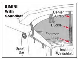
the soundbar. Push the end of the strap through until you can get ahold of the strap to pull the buckle through. Wrap the center strap inside the top around the sport bar, pull the strap forward to the windshield. Thread the strap through the footman loop on the windshield frame. Then pull the end of the strap back and thread it through the buckle. Tighten it securely.
