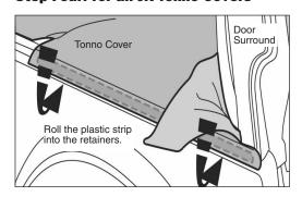
SECURE PLASTIC STRIPS ON SIDES Roll the plastic strip on each side of the Tonno Cover into the retainer channel on the vehicle.
