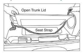
PLACE SEAT STRAP IN TRUNK Open the trunk and lay the Seat Strap across the bottom of the trunk.
