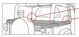
SECURE FRONT SPORT BAR STRAPS Wrap the straps on the front edge of the Tonno Cover around the B-Pillar sport bars and the bows. On each side of the
