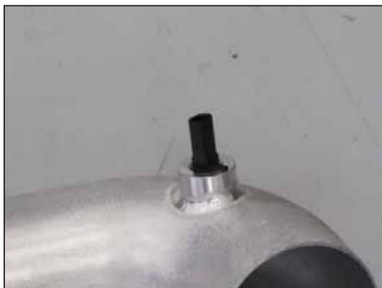
28. Install the inlet air temperature sensor into the K&N® intake tube as shown. **NOTE: Align the tab on the sensor with the line on the sensor mount then rotate clockwise to lock into position.**
