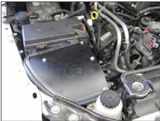
22. Install the K&N® filter lid and secure with the provided hardware.
