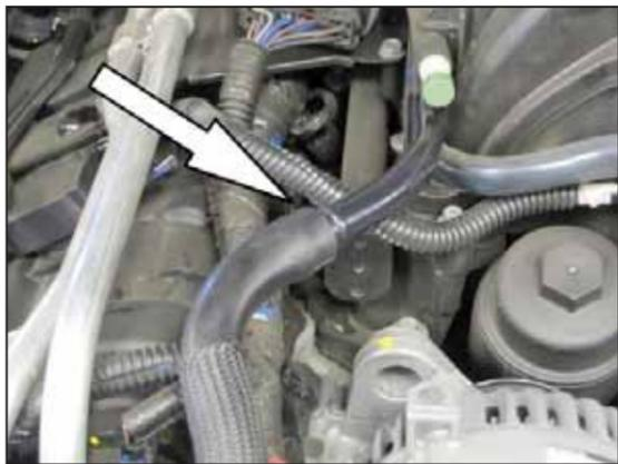
7. Disconnect the crank case vent hose from the crank case vent tube.
