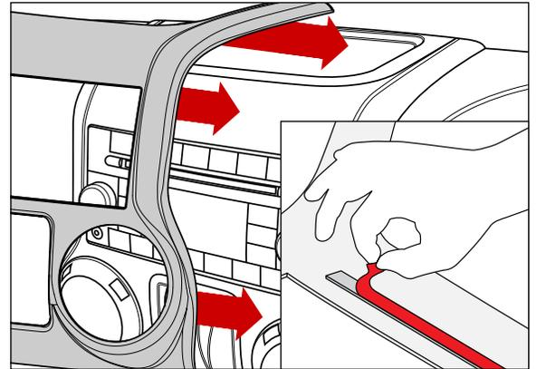
6. Firmly hold item in proper mounting position while pulling the exposed plastic liner to completely remove. Maintain pressure on installed item for 60 seconds to ensure proper contact. Full adhesion occurs within 24 hours of application.
