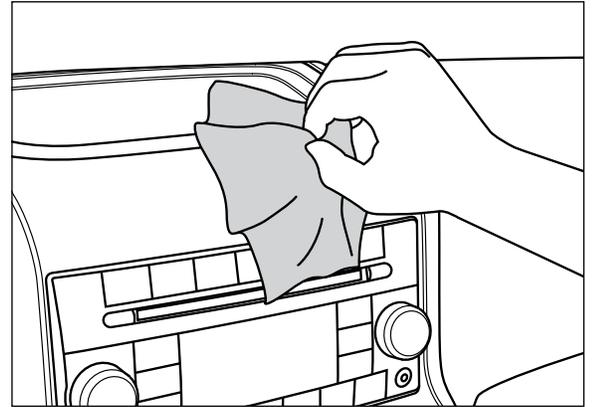
4. Remove only enough plastic liner to be easily gripped when item is installed.
