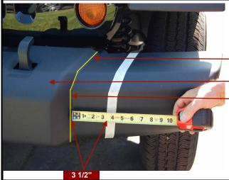
1) Measure 3 1/2" from the Bumper Pad toward the outside of the bumper both on the top of the bumper and the front of the bumper and mark with tape
