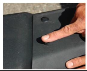
**5)** With the Holes aligned - Install the Black Plastic Pin Plugs pushing through the Bumper Cap into the holes in the bumper. You are now complete and the Bumper Cap is Installed.
