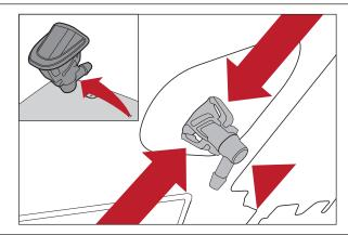
25. Attach washer fluid nozzle to JK Hood Vent . Make sure nozzle faces rear of vehicle.
