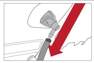
24. Compress and push washer fluid nozzle(s) outward to remove.
