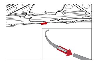
27. Attach supplied tube to washer fluid nozzle on your hood. Cut excess tubing if necessary.
