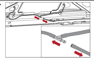
22. Separate washer fluid tube from spliced tubes connected to the nozzles.
