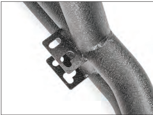
Figure 3: Carefully align the multiple mounting holes in the bumper with the frame mount holes to ensure proper fitment.
