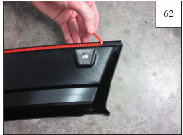
Pull back 1-2 inches of red tape liner from each end of installed edge trim and fold towards outside of the flare.
