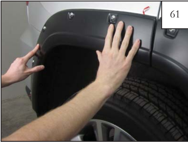
Hold Rear Main Flare up to wheel well to confirm fit. Do not install fasteners at this time.
