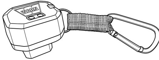
2. Plug the wireless receiver into "D" plug of control pack.
