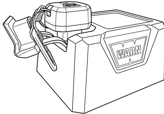
4. Remove receiver from winch when not in use.
