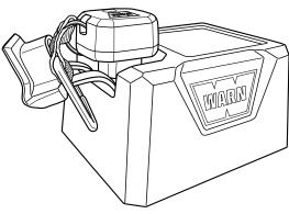
4. Remove receiver from winch when not in use.
