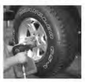
Remove all wheels and tires to make body lift installation easier 19 mm or 3/4socket
