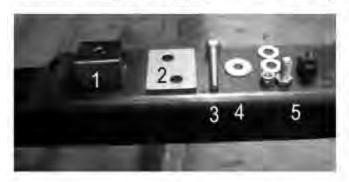
steering raise cube, goes on top of frame / under steering shaft
