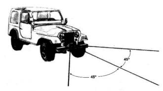
Winches equipped with cable guide fairleads can pull from several directions. Pull from an angle only to straighten up the vehicle-otherwise you can damage structural members or other parts of your vehicle and cause excess cable buildup on one end of the winch drum.
