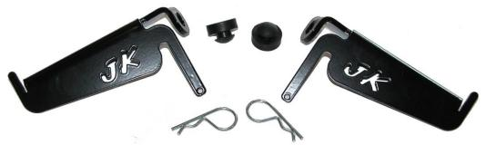
**Step 1:** Using a little liquid soap, push the rubber bumper into the hole on each foot peg. It's helpful to twist the bumper a little to get it into the hole.
