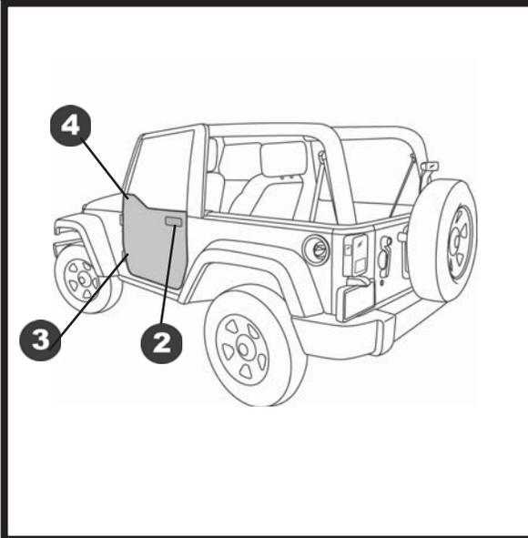
**NOTE** If the Element Door does not match up with the door striker, you may adjust the door striker by loosening it with a T-45 torx wrench and either lowering or raising the door striker. Tighten the door striker securely after adjusting. The door striker will have to be put back into its original position to reinstall O.E. doors
