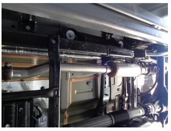
Step 3: Begin installation of your new MAGNAFLOW system by attaching the inlet assembly to the catalytic converter outlet using the OEM clamp. Keep all fasteners and clamps loose until final adjustment.
