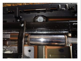
Step 3: Begin installation of your new MAGNAFLOW system by attaching the Resonator Assembly to the catalytic converter outlet using the OEM clamp. Engage the welded hanger to the rubbe insulators. Keep all fasteners and clamps loose until final adjustment.
