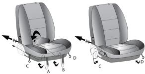
Step 1. Position cover over seat bottom. Pass flap between seat back and seat bottom. (Similar to the seat back cover installation, it may be easier if you fold the seat back forward) Join and tighten the buckles (A,B) under the seat.
