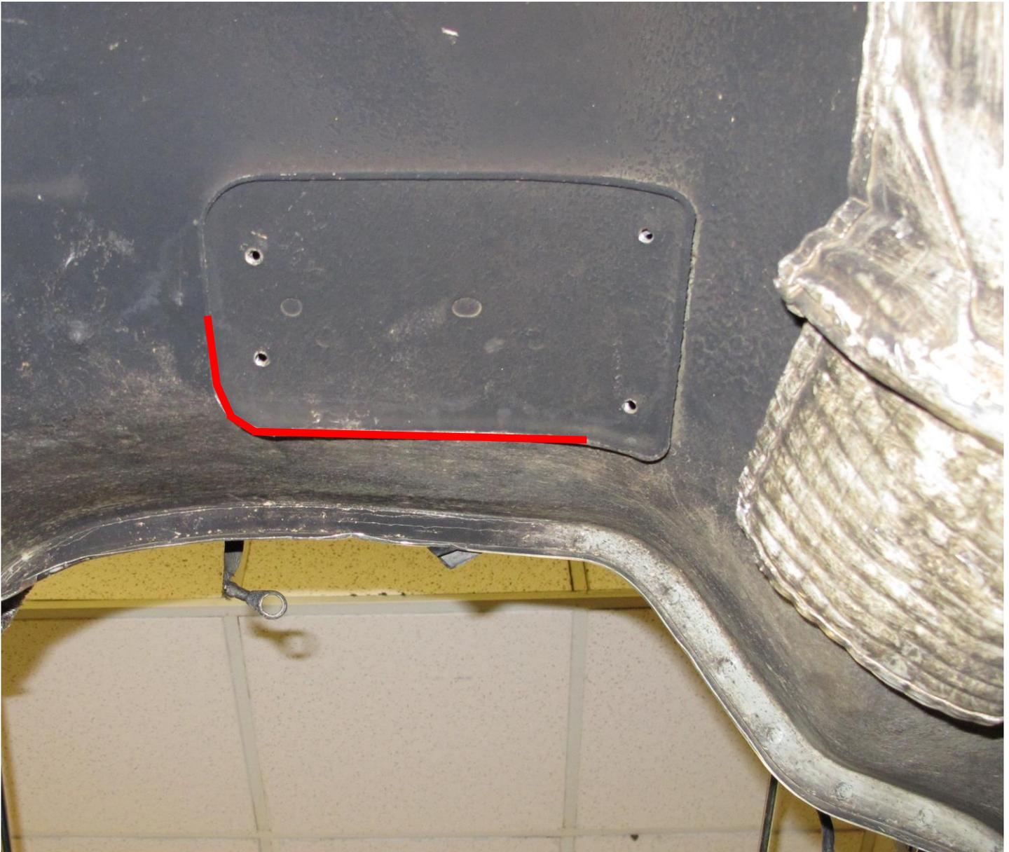
**Image 7- Air Bag Module Gusset Bracket Under Floor of Body Tub**
