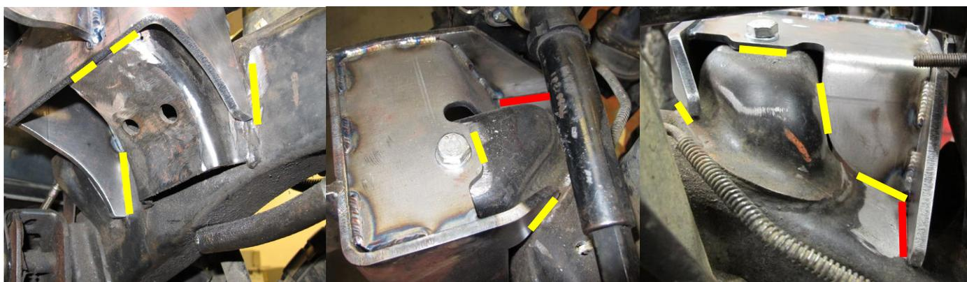
**Image 6 - Minimum Weld Locations for The Driver's Side Engine Mounting Bracket**
