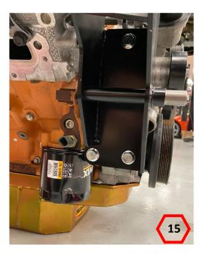
3. Next, loosely install the spacer and M8 x 1.25 x 50MM bolt into the top of the bracket.
