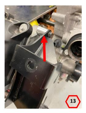
4. Torque each M10 x 1.5 bolt to 48 Ft. Lbs (65Nm) and the upper M8 x 1.25 to 21 Ft. Lbs (28Nm) following the below sequence.
