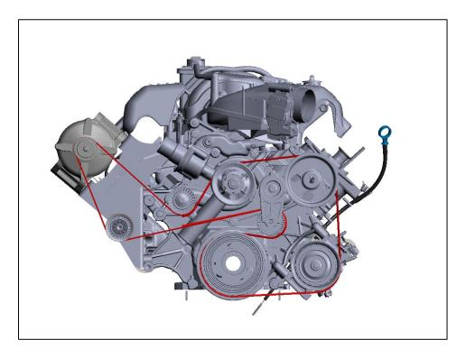
8. Attach all electrical connections to the alternator and start the engine. Observe the belt and ensure no slipping, binding, or excessive vibration is present. If the belt slips off, check to make sure you are using the proper idler pulley alignment position.
