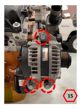
Clean the alternator mounting surface so that it is smooth and free of excessive corrosion. Using the supplied M10 x 1.5 x 25MM bolts, loosely install the Holley alternator bracket. NOTE: Do not tighten the bolts at this time.
