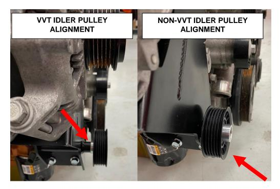
Inspect the assembly and ensure all hardware has been torqued to the proper specification. A longer belt is required since the alternator position has moved. Holley recommends using a 20mm x 2492mm belt, or 6K975. This belt can be found at most automotive parts retailers. Below is the proper belt routing.
