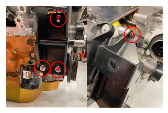
5. Next, install the OEM Chrysler alternator to the Holley bracket using the OEM bolts which were removed from the OEM bracket at step 1. Use the supplied flanged hex head locking nuts and torque the bolts to 48 Ft. Lbs (65Nm).
