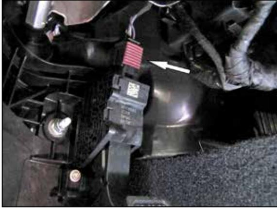
2. Release the locking tab and then disconnect the Throttle pedal electrical connection.
