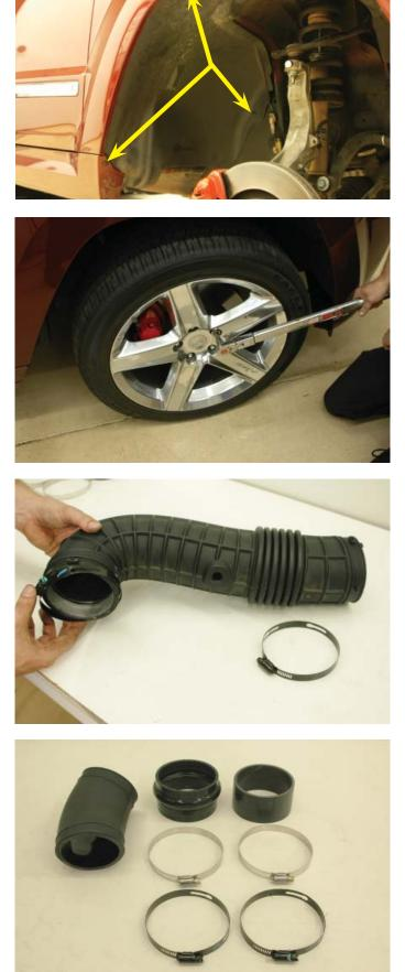
168. Mark and notch the supplied 'hump' hose to go past the two fins on the top of the OEM air box.
