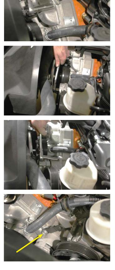
176. Attach the supplied idler bracket to the top water pump bolt location and the supercharger pulley support using the provided bolts. Torque to 20 ft lbs.
