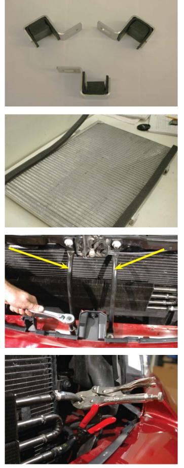
68. Use a drain pan to catch dripping fluid from the power steering cooler, and cut the two hose clamps holding the pinched hoses to the power steering cooler. Pull the hoses off the hose barbs of the power steering cooler, and pull the cooler off the plastic tabs mounting the cooler to the face of the air conditioning condenser. Set the power steering cooler aside for later reinstallation.
