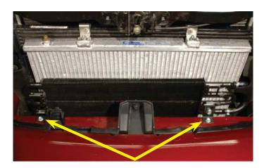
80. Re-attach the fascia braces on either side of the hood latch in their original location using the factory hardware and tighten securely.
