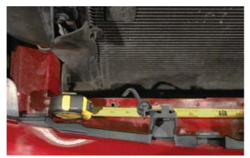
72. Slide the two carriage bolts into the slots of the intercooler heat exchanger and place the heat exchanger just in front of the air conditioning condenser on top of the bumper support. Use the location of the two bolts to locate where to place two of the prepared intercooler heat exchanger mounting brackets. Press the mounts into position on the air conditioning condenser top tank.
