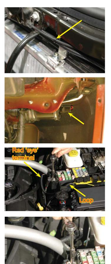
156. Remove the 25A fuse #43 for the coil-actuators from the rear fuse center.Verify using the owner's manual that you are removing the coil-actuators fuse.Do not rely on just the fuse number specified.
