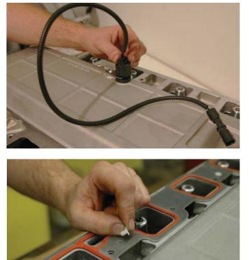
93. Inspect, and then install the OEM intake gaskets on the new supercharger intake manifold, press the locking tabs provided into the mounting holes to keep the gaskets in place. When finished flip the supercharger back over onto some blocks to protect the IAT sensor from damage.
