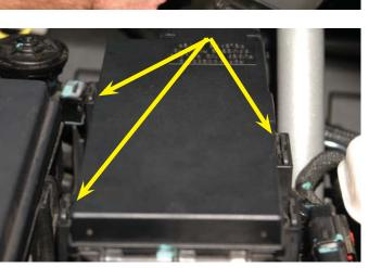
12. There is a wiring harness that has two clip locations that tie the harness to the fuse center mounting bracket. Pry these harness clips off of the fuse center mounting bracket.
