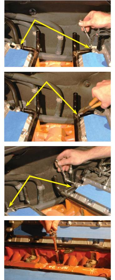
40. Use a 10mm wrench to remove the heater hard line mounting bolt from the water pump.
