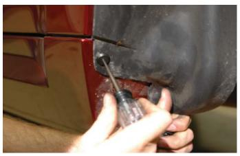
128. Remove the splash shield fender well from the vehicle and set aside to reinstall later.
