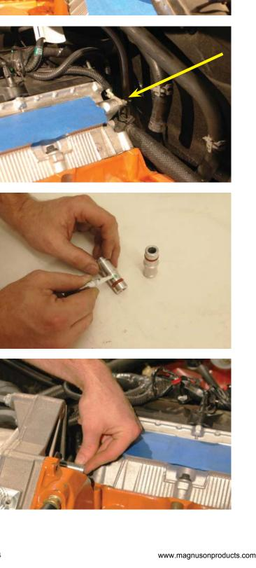
48. Use your fingers to press the other prepared barb into the driver side hole of the water pump that was vacated by the removal of the driver side hard line heater pipe that ran under the OEM intake manifold.
