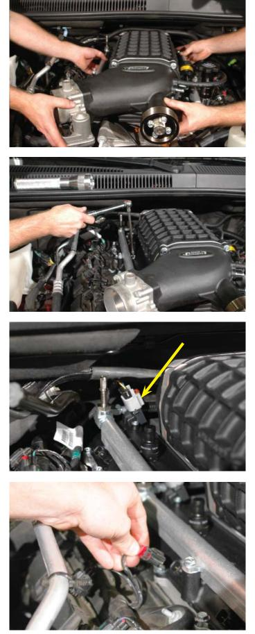
104. The IAT extension harness should be exiting below the supercharger intake manifold assembly on the passenger side of the engine. Connect the extension to the existing IAT plug and tuck the wires under the throttle body upon completion.
