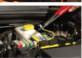
160. Route this wire over to the fuse tap just installed and plug the spade end onto the fuse tap. Bend the wire over toward the center of the box and close the cover.
