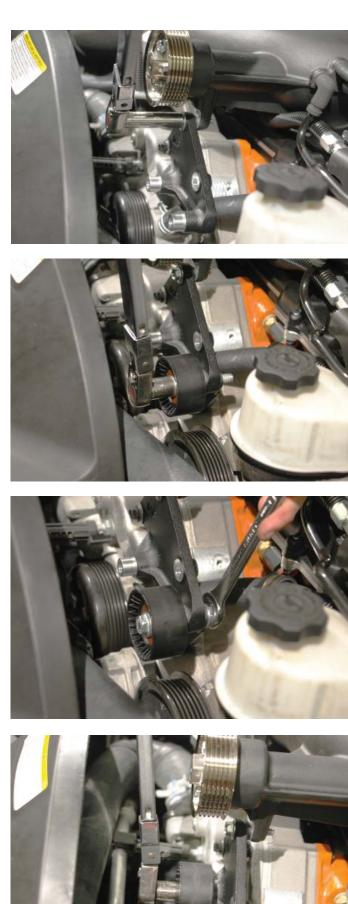
180. Torque the second water pump bolt (finger-tightened earlier) using a 13mm wrench and torque to 20 ft lbs. Always verify your torque wrench settings.
