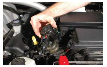
8. Open the cover of the forward fuse center just behind the battery on the driver side of the engine compartment, and un-snap the hinges from their posts to remove the cover. Set aside for later usage.
