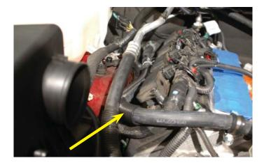
56. Cut about 1-1/2" from the end of the other heater hose at the firewall that used to run to the driver side hard line running under the OEM intake manifold.
