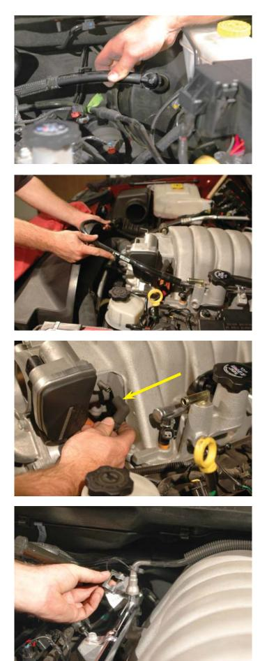
28. Use shop rags to catch residual fuel and the fuel line removal tool to disconnect the fuel line from the passenger side fuel rail. First press the fuel line further onto the fuel rail barb, then push the fuel line removal tool into the fuel line to release the locking clip. Now pull the fuel line free. We recommend plugging the fuel line and capping the fuel rail barb. Clean up residual fuel using shop rags and dispose of the contaminated rags properly.
