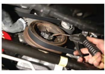
192. Once again blow out the holes and area to ensure all debris has been removed.
