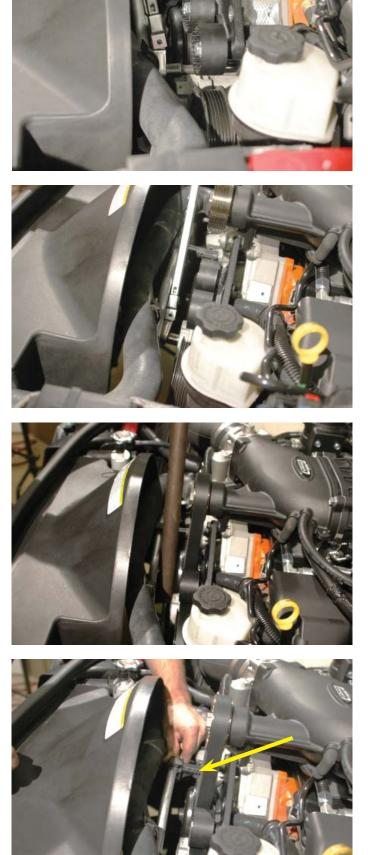
184. Remove the air box end of the hose from the OEM PCV plastic line and replace with the provided 4" section of 5/8" hose. Connect the remaining OEM hose end to the front oil fill spout hose barb and the new hose end to the air box end and air box. Secure to the air box using the provided spring clamp.
