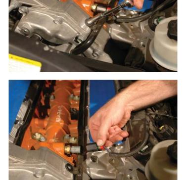
44. Replace the driver side ground sensor and ground wires to the head using the original stud. Clock the ground sensor toward the driver fender to gain the clearance necessary for the supercharger installation.
