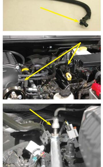
112. Extend the 'lobe' of the notch in the driver side coil pack cover approximately 1" further toward the rear of the cover and press in place over the coil packs in the original location. This modification is to create clearance with the oil separator drain hose to be installed next.
