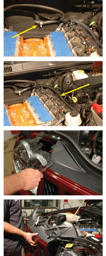
64. Cut strips of the supplied adhesive backed rubber and apply to the inside surfaces of the heat exchanger mounting brackets, on top of the strips applied, cut and add the  $\frac{1}{2}$ " adhesive backed rubber as shown.
