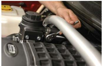
147. Connect the hose from the driver side barb of the supercharger intercooler to meet the hose from the intercooler pump inlet barb. Cut the hoses to fit and connect together using the provided coupling (hose mender), and secure in place using the provided spring clamps.
