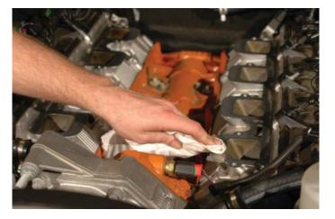
100. With the help of an assistant, set the supercharger assembly in place. Be careful with the protruding bolts and the IAT sensor harness wires which must exit below the assembly toward the front of the supercharger on the passenger side.
