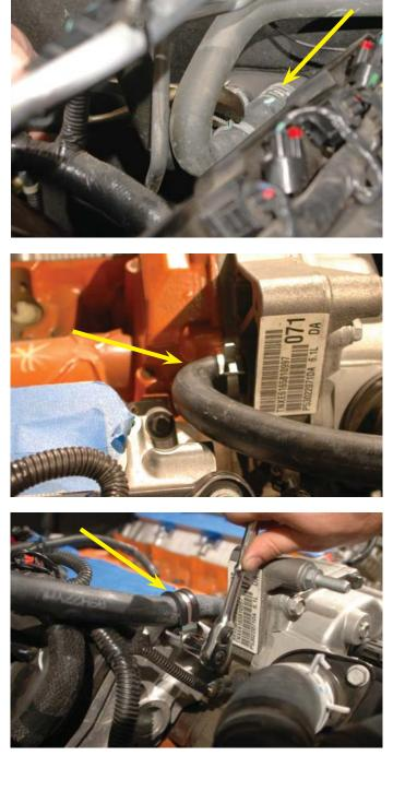
52. Install the supplied  $\frac{3}{4}$ " -5/8" coupling (hose mender) in the supplied  $\frac{3}{4}$ " x 7" section of hose. Secure in place with a supplied spring clamp.
