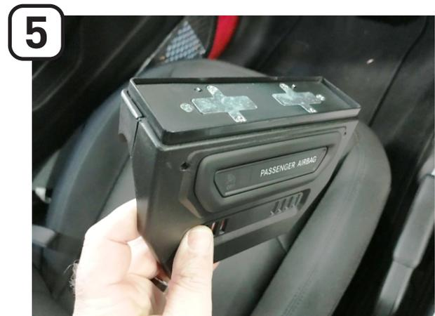
Install the warning lamp into the Trigger overhead mount by inserting into the opening until the metal tabs snap in place. Then plug the connector back into the lamp.
