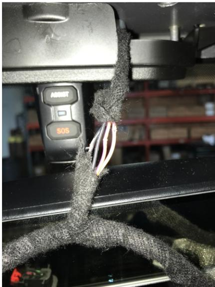
If running the optional 12V power to the RF remote, open up the factory rear view mirror harness and locate the black wire for ground (attach black wire from 12v harness) and the Orange/Pink for keyed ignition (Red and white wires from 12v harness) . Use wire splices or a preferred method to tie into the wires. **NOTE: Use this as a guide, our example was an early production vehicle, always test the wires before connecting.**
