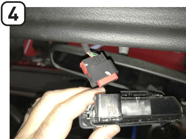
Press on the top of the red tab (closest to the wires) to release connector to the warning lamp.
