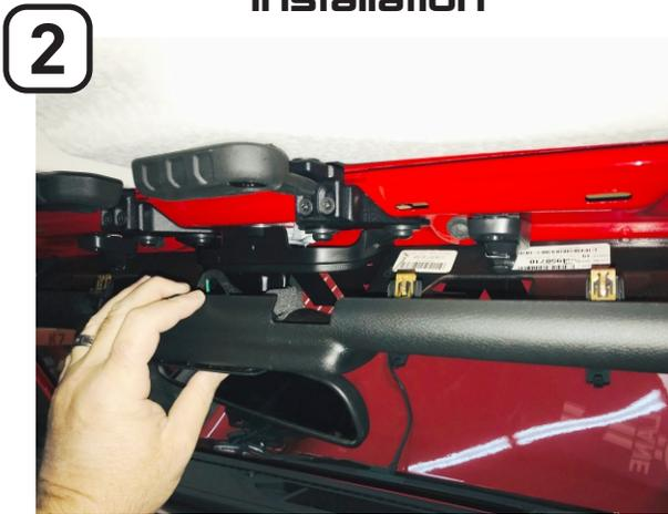
Start by pulling down firmly on the front of the factory header shroud to expose the wiring and connector for the warning lamp.
