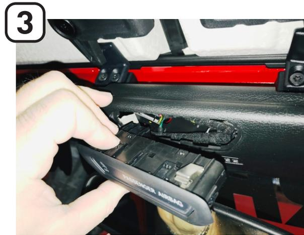
Press in on the metal tabs holding the warning lamp into the header shroud and remove lamp.
