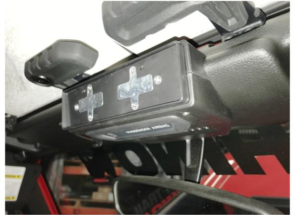
**NOTE:** If installing the 12V power cord, route the cable through the opening for the warning lamp in the factory plastic header shroud.
