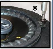
Screw speakers to pods with the included #10 X 3/8" screws
