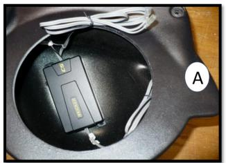
**A:** Crossovers can be placed inside the pods. We dropped one in the driver's side pod to show the best mounting orientation (driver's side pod shown).
