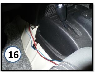
Bring the Remote and Amp Power wires under the carpet, between driver seat and center console so they can come up from under the carpet under the driver seat. You can bring them up where the other factory wiring for the seat exits, or cut slits in the carpet exactly where they will need to be for the amp.
