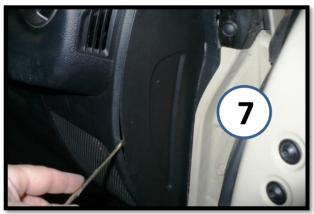
**Amp Power Wire:** Pop off this little side panel on the passenger side dash with a flathead screwdriver. It pops off easily. (This is the panel in later models).
