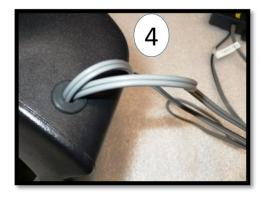
Insert grommet w/ wires into hole in pod. Push through from outside while pulling grommet from inside and you'll be able to get it through and inserted properly as shown. Keep only enough wire inside the pod to connect to the woofer and tweeter. Here's where you may want to use a glue gun or wax, etc. to fill any gaps around the wires so air can't escape the pod. Not absolutely necessary, but if you get a whistling sound, this is likely why.
