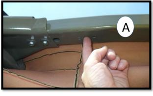
In these photos with the foam piece removed, you can see where the screws will enter the sport cage on the driver side. (Mirror image for passenger side.)
