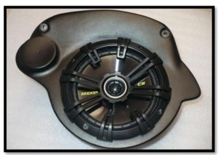
For those installing their own coaxial speakers with no separate tweeters, you'll simply leave the tweeter sections uncut and install your coaxial speakers similar to the Kicker Coaxial shown in the photo here.
