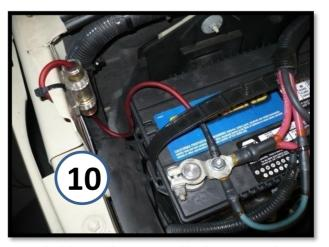
Fuse holder can be mounted by battery as shown.
