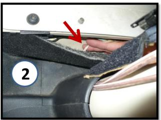
Pulling the carpet back, you can grab the wires as they're fed under the plastic piece at the base of the sport bar.
