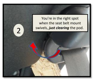
With the ½" wood spacer in place, you can tell the pod is at the correct angle when the seat belt guide (shown) can swivel past the pod, missing it by just a little bit. (If it's missing it by more than ¾" you need to swing the pod forward). This ensures the first screw goes in at the right spot!
