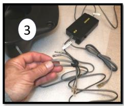
Then push the labeled 'Mid' wires through the grommet *in the opposite direction*. It's a tight fit but that minimizes air escaping the pod.
