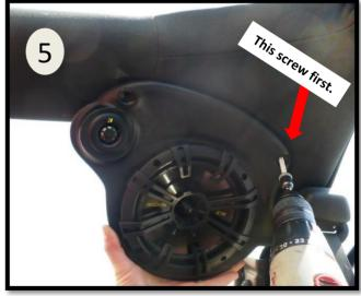
Installation is easier if you first feed the speaker wire behind the fabric, especially if you made the fabric slit.
