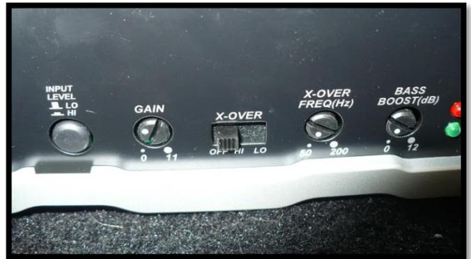
For Kicker amp, this is how we ended up setting ours: Stock 130 radio in our Jeep so input level is on High and we tapped into the sound bar speakers. We put the gain about a third of the way up and kept the x-over off so the pods get the full audio spectrum. We had the bass boost down/off. We had our regular stock 130 radio set at +4 bass, +1 treble, +2 mid, balance centered and fader at +4 Front. It's at least a good starting point for you if you got the Kicker amp too.
