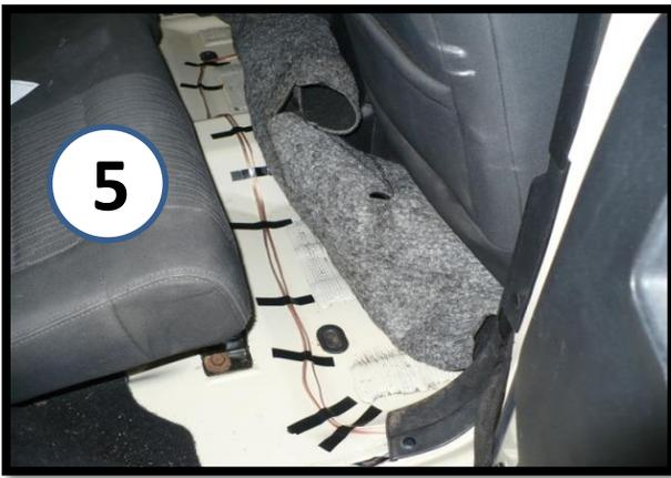
Now run the wires over to where the amplifier will be installed under the driver seat. If using your own amp, it will have either a **High Level Input** with a small plug of wires, or a High/Low Level button the wires will connect to using RCA adapters. Consult the manual for your amp.
