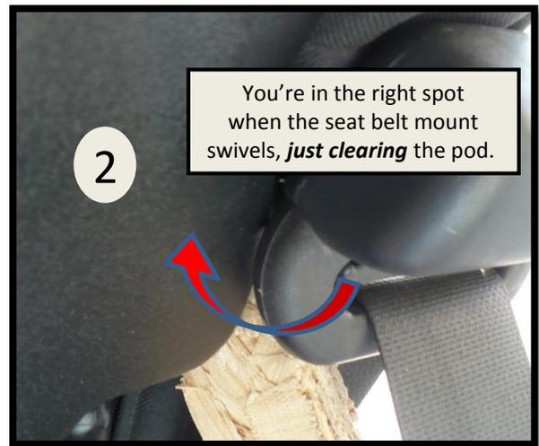
With the ½" wood spacer in place, you can tell the pod is at the correct angle when the seat belt guide (shown) can swivel past the pod, missing it by just a little bit. (If it's missing it by more than ¼" you need to swing the pod forward). **This ensures the first screw goes in at the right spot!**
