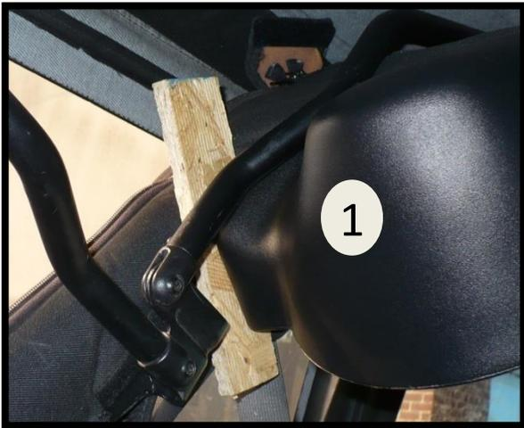
**Getting a feel for where it will go** - use a small piece of wood that's ½" thick to show how close the JKU-Pod should be to the downward sport bar. Place the wood as shown in the photo so it spans that side of the pod appropriately. Wood piece should butt up against fabric & metal; any factory wiring under the fabric should be moved aside.
