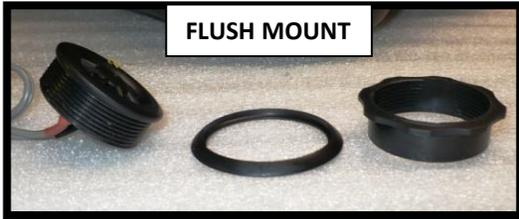
You need to pick a mounting configuration (flush mount or angled). Shown here are the Kicker tweeter, trim ring, and shorter mounting nut needed for a **flush mount** scenario.
