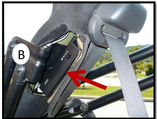
**B:** Using a couple of zip ties could provide a place for the crossovers behind the hook & loop opening in the fabric for the soft-top bars.
