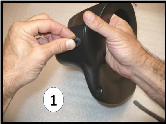
Insert your rubber grommet. This is where the wires will exit the pod.
