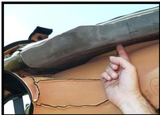
These two photos show you where the screws will penetrate the foam and affix the driver side pod. (Think mirror image for the passenger side.) The foam can sort of jiggle around, but that goes away when the pods are installed.
