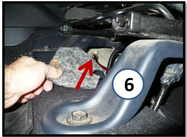
**Amplifier Ground:** An easy connection is already right under the Driver seat. It's up by the inner seat bracket on the uphill slope of the floor. Use 10mm wrench to loosen the nut and use a ring terminal on the ground wire. Ground Wire must be connected to amp prior to attaching Power or Remote Wires to amp!
