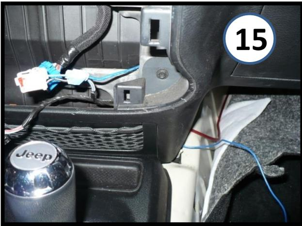
'11-'18 Feed remote wire down behind dash to meet up with power wire and run remote wire under dash to driver side area just like power wire was done. Note: if you're adding other amplifier(s) for other audio upgrades, you only need to run this single Remote wire over to the amp(s) and can then splice into it for additional short runs to the other amp(s).
