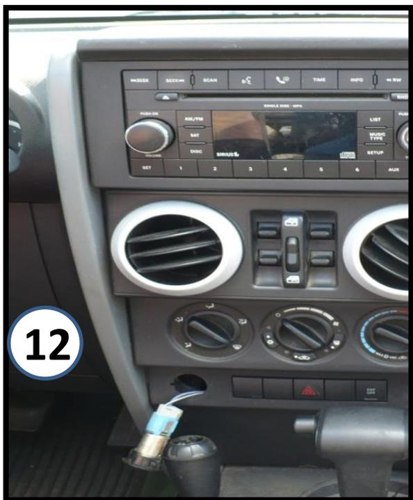
'07-'10, pop out the cigarette lighter housing on the left using a small pick or tiny flathead- the tabs right behind the face can be pushed in to pop it out.
