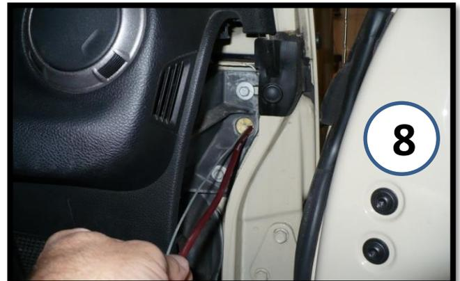
Behind it is a little hole that has foam in it. Use a piece of wire such as a coat hanger with the power wire taped to it and poke it through.
