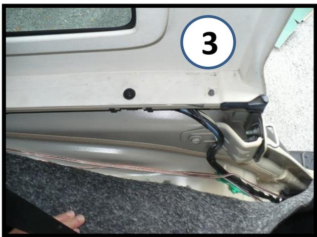
Continue running the speaker wires under the carpet along the driver side wheel well. Bring them under the rear floor carpet until you get under the driver seat. They can exit at seat bracket or you can make a slit in carpet at the exact spot where they'll connect to the amp.
