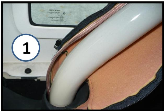
You must run two sets of speaker wires from the pods to your amplifier. Make note of which are left, right and pos.+ and neg. – so you know which is which up at the amp. Start with the passenger side pod: unzip the sport bar fabric to slip the wire underneath. When it's over by the driver side pod, start a second run of wire for the driver side pod and bring both pairs together down the sport bar as shown here.
