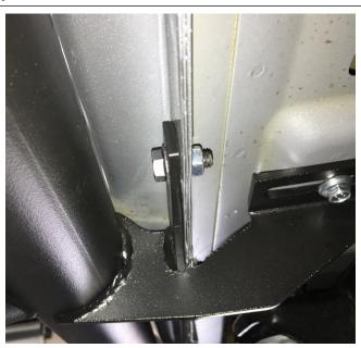
**Step 6.** Continue installing the rest of the hardware in the remaining brackets and leave loose.
