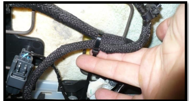
A cable tie can hold the excess wire lengths to the spring work of the seat bottom, ( check for full seat slide ability front to back ).
