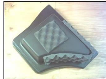
Simultaneously push the pod back, toward the floor, and to the rear of vehicle and then run the self-tapping screws in order as shown:
