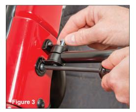
Use a 12mm wrench and socket to remove the nut and lock washer and partially remove the bolt as shown
