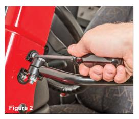
**Step Three: Install Mirror Bracket** Start with the top screw first. As shown in FIG2, Install the supplied T40 button head cap screws and washers to affix the mirror bracket to the vehicle using a T40 head screwdriver.
