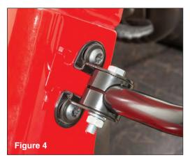
while tightening the torx screw with and T40 screw driver. Reinstall the lock washer and nut and snug (FIG4).
