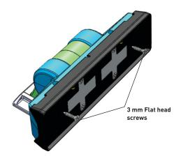
Installation of Trigger Mounting Plate
