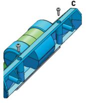
Install the 2 screws/washers for the pivot loosely into the pivot hole as shown. Now install the lower half of the main mount (C) being careful to be sure the washers are in the correct location.
