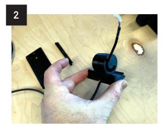
Halves are then screwed together with wire inserted. Use the 2.6 mm pan head screws.
