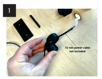
If running 12 volt power to the Pedestal, insert the 12 volt power wire included in the original Trigger 6 Shooter packaging (not included with Pedestal Kit). Wire is inserted on one side of the base, then routed through opening as shown.
