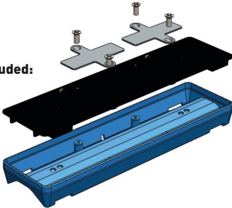
Begin assembly by removing the inner plate of the original Trigger mount included with the Trigger 6 Shooter kit. Remove the four screws and set aside with the top plate/wire/connector, all will be re-used for the visor mount.
