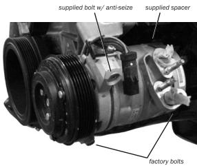
14. Install the starter (torque to 40 ft/lbs), modified A/C compressor (torque to 18 ft/lbs), and the engine idler pulley (torque to 40 ft/lbs).
