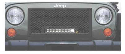
**STEP 4** - Re-install the front fascia by inserting the turn signals back into place and re-connecting them. Push the bottom clips back in place along with the clips along the top.
