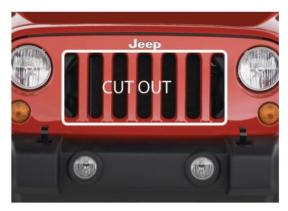
*STEP 3* - Before installing the new grille, install the LED bar and tighten securely. Ensure the LED cable is fed to a location that can easily be reached for connecting to the harness after the grille is in place. Lay the new grille in place and attach the provided brackets to the back of the grille and tighten.
