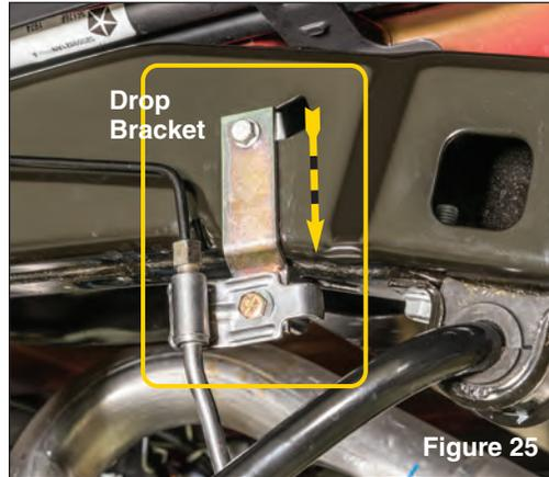
and open end wrench. (see FIG 24) Install brake line drop brackets using the original bolt to the frame, and the supplied 1/4" fine thread bolts, washers and locknuts as shown with a 7/16" socket and open end wrench. (see FIG 25)
