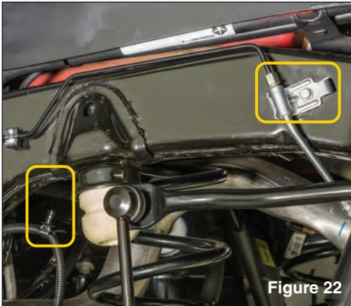
Disconnect ABS line from frame and disconnect brake line from frame using a 10mm socket. (see FIG 22)
