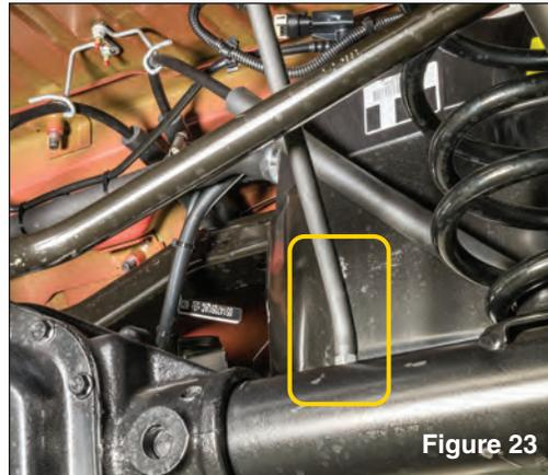
Disconnect axle housing vent line. (see FIG 23)
