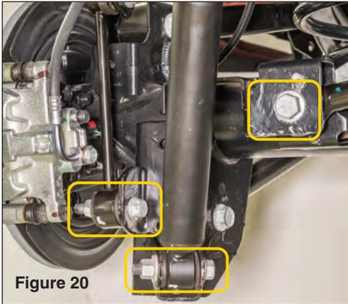
**Moving to the rear of the vehicle:** Raise rear end and properly support using jack stands. Disconnect the rear track bar bracket from axle using 21mm socket, remove rear lower shock bolts and sway bar end links using a 18mm socket and open end wrench (FIG 20).
