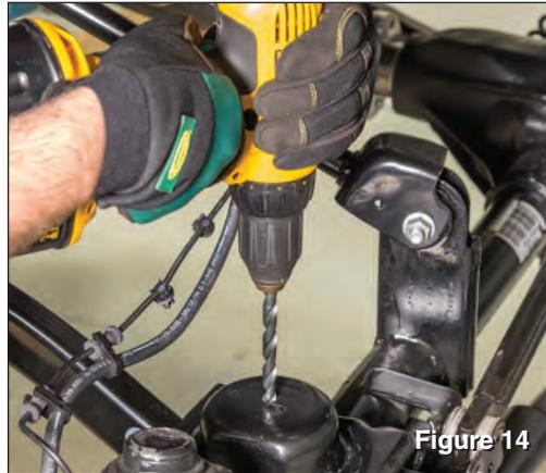
Locate the new front bump stop in the kit. Using the bump stop as a template, mark the center of the bump stop pad located on the front axle. Consider drilling pilot holes. Carefully drill the bump stop pad using a 25/64" drill bit. (See FIG 14).
