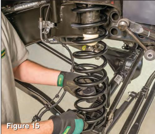
With axle in drop position, place bump stop in coil springs, and position the new coil springs.
