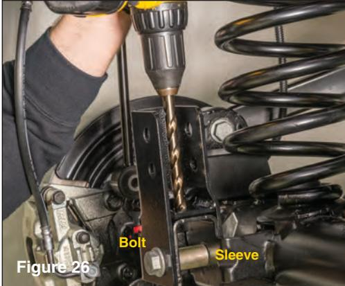
Place supplied rear track bar bracket over axle housing. Install OEM bolt and crush sleeve, but do not tighten at this time. Carefully drill a hole through the track bar bracket into axle housing bracket as shown using a 15/32" drill bit. Consider drilling pilot holes. (see FIG 26)
