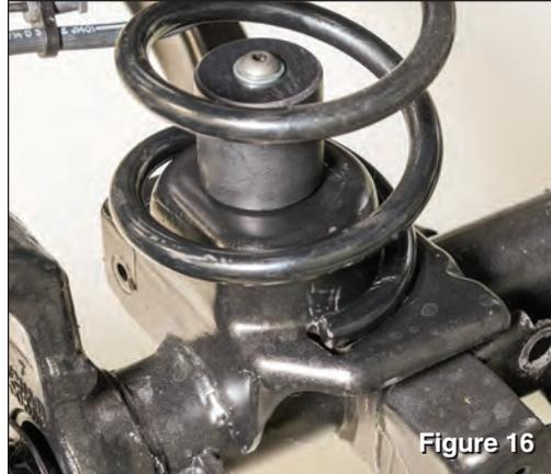
Attach bump stop to axle using the 10mm button head bolts and one washer under the 10mm nut, as shown (see FIG 15&16). Perform this on both sides of the vehicle.
