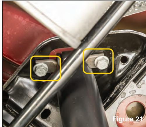
Now disconnect the top end shock bolts shown above using a 16mm socket. (see FIG 21).
