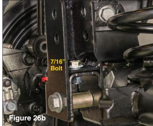
Install supplied 7/16" fine thread bolt, and washer into the hole you have just drilled. Secure from the underside with the supplied locknut, do not tighten at this time. (see FIG 26b)
