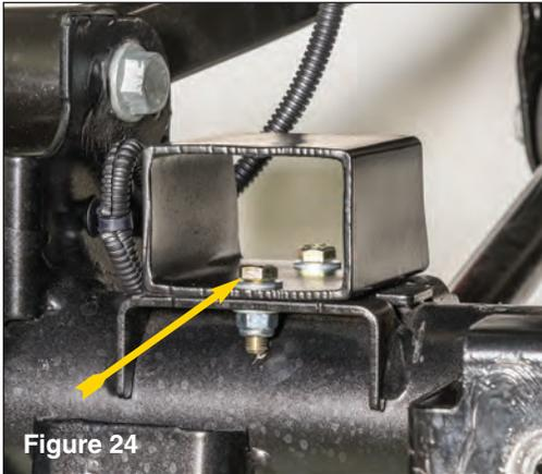
Safely lower the rear axle in order to remove the original equipment rear springs. Install the new coil springs in position. Gently raise axle to hold new springs in place. Install new bump stops with 5/16" fine thread bolts, washers and locknuts as shown using 1/2" socket
