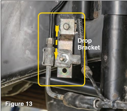
For '07-'10 model years only: Using a 7/16" open end wrench and socket, install brake line drop brackets and separate ABS line from top of brake line using 1/4" fine thread bolts, washers and locknuts as shown. (see FIG 13)
