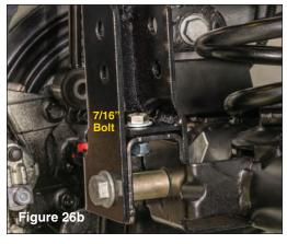
Install supplied 7/16" fine thread bolt, and washer into the hole you have just drilled. Secure from the underside with the supplied locknut, do not tighten at this time. (see FIG 26b)
