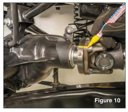
Mark the front drive shaft position with a paint marker and remove 4 bolts using a 15mm socket. (see FIG 10)
