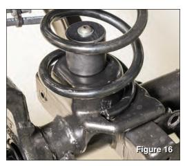
Attach bump stop to axle using the 10mm button head bolts and one washer under the 10mm nut, as shown (see FIG 15&16). Perform this on both sides of the vehicle.
