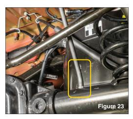
Disconnect axle housing vent line. (see FIG 23)
