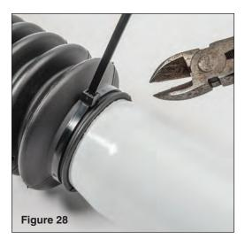
Assemble your new rear shocks as shown in FIG 28, 29 & 30. Install the shock boots and secure with zip-ties. Clip off zip-tie tail. (see FIG 29).
