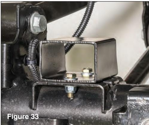
Install new bump stops with  $\frac{5}{16}$ " fine thread bolts, washers and locknuts as shown using  $\frac{1}{2}$ " socket and open end wrench. (see FIG 33)
