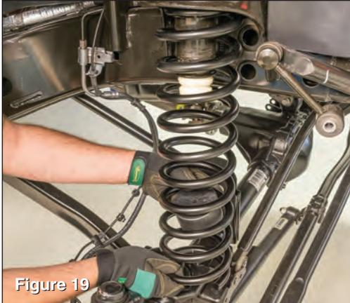
With axle in drop position, place bump stop in coil springs, and position the new coil springs. (see FIG 19 & 20)
