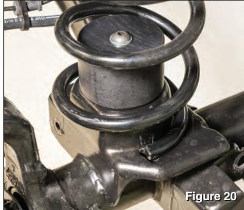
Attach bump stop to axle using the 10mm button head bolts and one washer under the 10mm nut, as shown (see FIG 19 & 20). Perform this on both sides of the vehicle.
