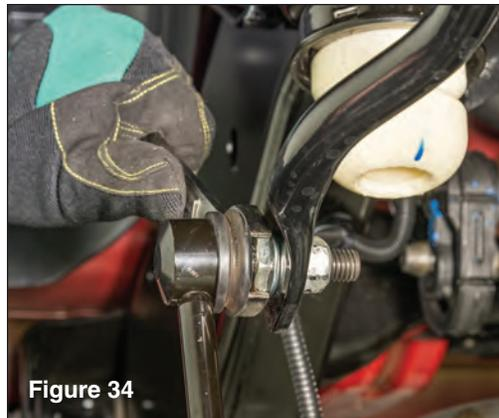
Using a 19mm open end wrench and 18mm socket remove rear sway bar end links and after rear work is complete, relocate these to the front of vehicle. (see FIG 34 & FIG 1)
