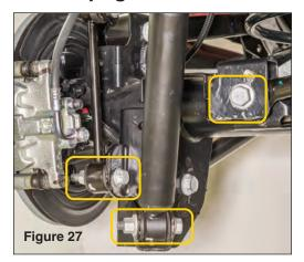
Moving to the rear of the vehicle: Raise rear end and properly support using jack stands. Disconnect the rear track bar bracket from axle using 21mm socket, remove rear lower shock bolts and sway bar end links using a 18mm socket and open end wrench (FIG 27).
