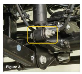
Disconnect the bottom end of the front shocks using an 18mm socket and open end wrench. (see FIG 3)
