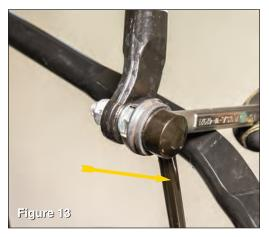
Using a 19mm open end wrench and 18mm socket remove front sway bar end links and discard. Your original equipment rear swaybar endlinks will be used in their place. (see FIG 13)
