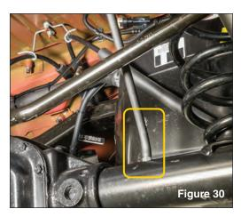
Disconnect axle housing vent line. (see FIG 30)
