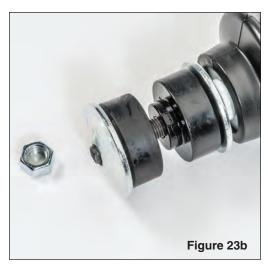
Assemble the shock top bushings exactly as shown (see FIG 23).
