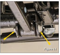
Locate front lower axle housing control arm mounting bolt and remove using a 21mm socket and open end wrench. (see FIG 14)
