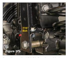
Install supplied 7/16" fine thread bolt, and washer into the hole you have just drilled. Secure from the underside with the supplied locknut, do not tighten at this time. (see FIG 37b)
