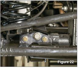
Install front track bar bracket using OEM bolt loosely at this time along with  $^{7}/_{16}$ " x 2  $^{1}/_{2}$ " fine thread bolts, washers and locknuts using  $^{5}/_{8}$ " socket and open end wrench. (see FIG 22)
