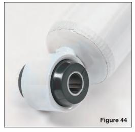
Assemble the shock bottom bushings exactly as shown (see FIG 44).
