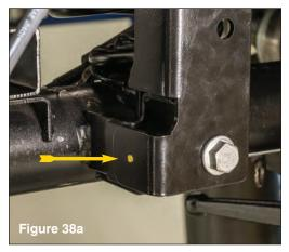
Mark location on the center of the new bracket face with paint marker as shown (see FIG 27). Consider drilling a pilot hole. It will be necessary to carefully drill through the drivers side of the new bracket and the axle housing mount using a 17/32" drill bit.
