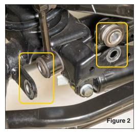
this time. Remove front tires/wheels. Disconnect the front sway bar end links using a 18mm socket and open end wrench. Disconnect front track bar using a 21mm socket. (see FIG 1 & 2)
