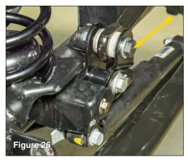
Re-attach track bar using a 7/8" socket and open end wrench with 9/16" x 3" coarse thread bolt, washers and locknut and torque to 111 ft lbs. (see FIG 26)
