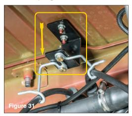
Safely lower the rear axle in order to remove the original rear springs. Install the new coil springs in position. Gently raise axle to hold new springs in place. Remove factory emergency brake cable retainer using a 10mm socket. Install the supplied drop bracket using ¼" x 1 fine
