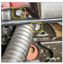
Install the top end of the new rear shocks using a 16mm socket.
