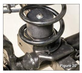
Attach bump stop to axle using the 10mm button head bolts and one washer under the 10mm nut, as shown (see FIG 19 & 20). Perform this on both sides of the vehicle.
