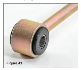
Assemble new rear extended sway bar links using supplied bushings and sleeves. (see FIG 41)
