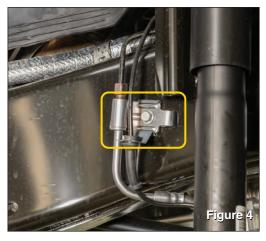
Disconnect brake line bracket from frame using a 10mm socket. (see FIG 4)
