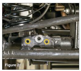
Locate front axle housing track bar mount and drill-out the two outer holes to  $\frac{7}{16}$ ". (see FIG 21)
