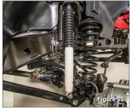
As shown in FIG 25, Install the top end of the new front shocks using a 9/16" open end wrench. Using factory hardware, re-attach bottom end of shock and torque to 56 ft lbs.
