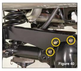
Loosely install brace with supplied <sup>5</sup>/<sub>16</sub>" coarse thread bolts, thick washers and lock washers using a <sup>1</sup>/<sub>2</sub>" socket. (see FIG 40)
