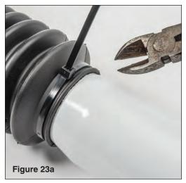
Assemble your new front shocks as shown in FIG 23a, 23b & 23c. Install the shock boots and secure with zip-ties. Clip off zip-tie tail.
