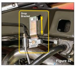
thread bolts, washers and locknut. (see FIG 31) Install brake line drop brackets using the original bolt to the frame, and the supplied ¼" fine thread bolts, washers and locknuts as shown with a 7/16" socket and open end wrench. (see FIG 32)
