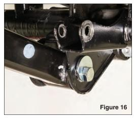
On each side, install new cam bolts and tighten to 125 ft lbs. (see FIG 16).
