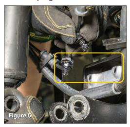
On 2011 and newer models disconnect the ABS lines from brake line bracket (see FIG 5)
