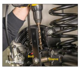
Place supplied rear track bar bracket over axle housing. Install OEM bolt and crush sleeve, but do not tighten at this time. Carefully drill a hole through the track bar bracket into axle housing bracket as shown using a <sup>15</sup>/<sub>32</sub>" drill bit. Consider drilling pilot holes. (see FIG 37)
