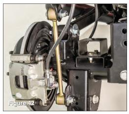
Install new links with supplied ½" button head bolts, larger washers under head of bolt, small washers under nut and locknut using a 5/16" allen wrench and 19mm socket. (see FIG 42)
