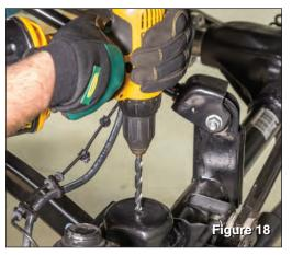
Locate the new front bump stop in the kit. Using the bump stop as a template, mark the center of the bump stop pad located on the front axle. Consider drilling pilot holes. Carefully drill the bump stop pad using a <sup>25</sup>/<sub>64</sub>" drill bit. (see FIG 18)
