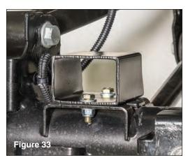
Install new bump stops with 5/16" fine thread bolts, washers and locknuts as shown using ½" socket and open end wrench. (see FIG 33)
