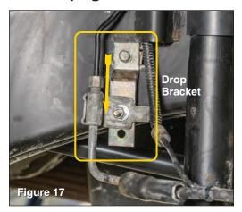
For '07-'10 model years only: Using a 7/16" open end wrench and socket, install brake line drop brackets and separate ABS line from top of brake line using ¼" fine thread bolts, washers and locknuts as shown. (see FIG 17)
