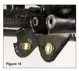
Using a punch and hammer, remove the knock-outs on either side of mounting hole surfaces, transforming each hole into a slot. (see FIG 15)
