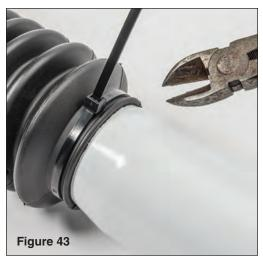
Assemble your new rear shocks as shown in FIG 43, 44 & 45. Install the shock boots and secure with zip-ties. Clip off zip-tie tail. (see FIG 43).
