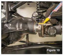
Mark the front drive shaft position with a paint marker and remove 4 bolts using a 15mm socket. (see FIG 10)
