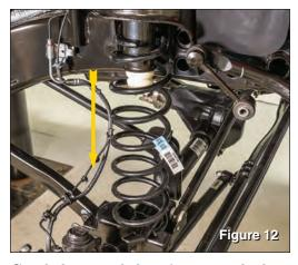
Gently lower axle housing towards the ground and remove original coil springs. (see FIG 12)
