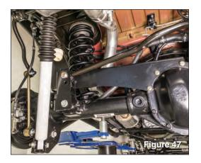
Finally, raise the axle using a floor jack so the full weight of vehicle is on the new coil springs.
