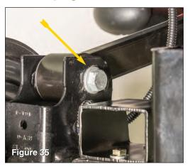
Locate rear upper axle housing control arm mounting bolt and remove using a 21mm socket and open end wrench. (see FIG 35)
