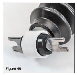
Push the mounting plate with bushing through the top eyelet of the rear shocks (see FIG 45).
