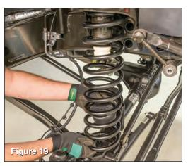
With axle in drop position, place bump stop in coil springs, and position the new coil springs. (see FIG 19 & 20)
