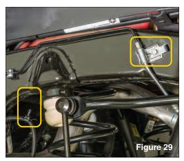
Disconnect ABS line from frame and disconnect brake line from frame using a 10mm socket. (see FIG 29)
