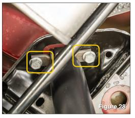
Now disconnect the top end shock bolts shown above using a 16mm socket. (see FIG 28).
