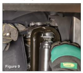
Disconnect the top end of the front shocks using two 5/8" open end wrenches. (see FIG 9)
