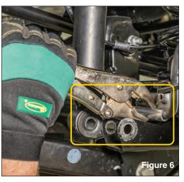
Using locking pliers, separate the bracket from brake line (FIGS 6 & 7).
