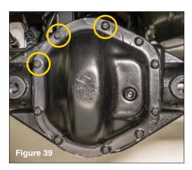
Locate the 3 differential cover bolts that will be removed for track bar brace installation. (see FIG 39)
