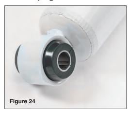
Press in the bottom end bushings as shown (see FIG 24).
