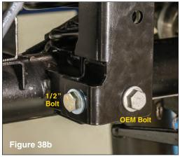
Install supplied  $\frac{1}{2}$ " x  $1^{1}/_{4}$ " fine thread bolt, washer and locknut loosely at this time. Tighten OEM track bar bolt followed by the  $\frac{7}{16}$ " and  $\frac{1}{2}$ " bolts.
