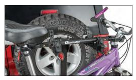
Adapter takes the place of a traditional top tube, allowing standard bicycle rack installation.
