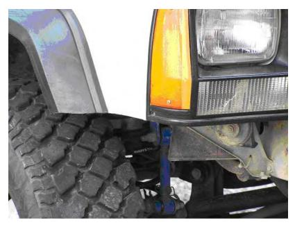
Time to cut the fenders: (only 96 and earlier require fender trimming.) I used a pneumatic cut off wheel. I made a straight cut starting at the headlight bezel and extending straight back to the fender flare. You can use whatever your preference is to cut sheet metel. It's best to use masking tape over the area to be cut to protect the finish and as a clean surface to mark the line.
