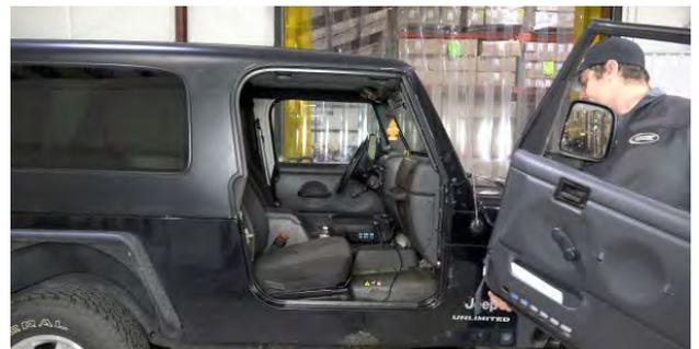
Lift your door straight up to remove the pins from the hinges. You may need to rock the door back and forth to get it to lift out. Store your doors in a safe place against a blanket or cardboard to protect the paint.
