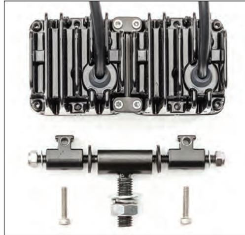
*Install the mounting feet on either side of the mounting bracket with a rubber washer on the inside and a flat washer and nylock nut on the outside. Tighten the Nylock nuts loosely using a 10mm wrench or socket. Install the mounting feet and bracket back into their original location on the Cube lights with the original cap screws and tighten with a 3mm hex wrench.*
