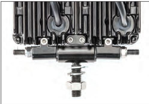
*At this point tighten all of the fasteners but take care not to overtighten. The bracket and lights can now be mounted and secured in place using the single mounting stud. Tighten the nut with a 17mm wrench.*
