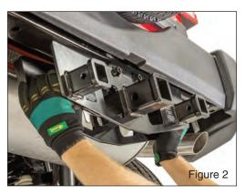
cross member, then install the 4 supplied bolts through the hitch and rear cross member and thread them into the weld nuts on the VersaHitch<sup>®</sup>
