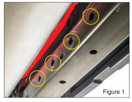
**Put on safety glasses.** Locate the four bolt holes in the rear cross member of your vehicle behind the Rear bumper. Install the VersaHitch<sup>®</sup> over the rear
