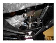
1) Place a provided clamp onto the slip-fit of inlet pipe assembly **#710TBS** and slide over the back of the factory Y-pipe. Connect the hanger on the pipe to the rubber mount on the vehicle and tighten the clamp enough to hold, but still allow for adjustment. The hanger closest to the slip-fit is for 07-11 models, the other hanger is for the 2012-2013 model. You may choose to trim off the hanger that is not used.
