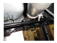
4) Place a provided clamp onto the slip-fit of exit pipe **#86127S** and slide onto the back of over-axle pipe **#86126S**. Connect the hanger on the pipe to the rubber mount on the vehicle and tighten the clamp enough to hold, but still allow for adjustment.
