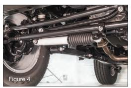
After installation be sure to cycle steering and check for adequate clearance. In most cases it will be necessary to rotate the stabilizer bracket on the tie rod down slightly to allow for clearance.
