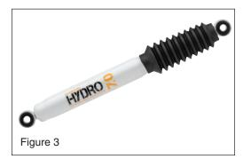
Install supplied boot over new stabilizer and secure using the boot tie. Install one supplied hourglass bushing and sleeve at each end of stabilizer. (see FIG 3)
