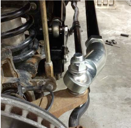
Passenger side knuckle connection
