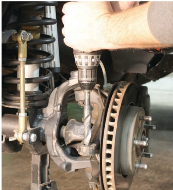
Drilling out knuckle to 18mm
